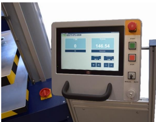
BCT control interface
