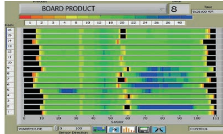
Dryer exit visualization shows the moisture profile of every board. As shown above, the wetter region indicated in blue on the right-lower mid decks could result in inconsistent board quality.
