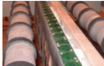
Each IMPS-4400 features an array of RF sensors that span the width of the entire board line.
