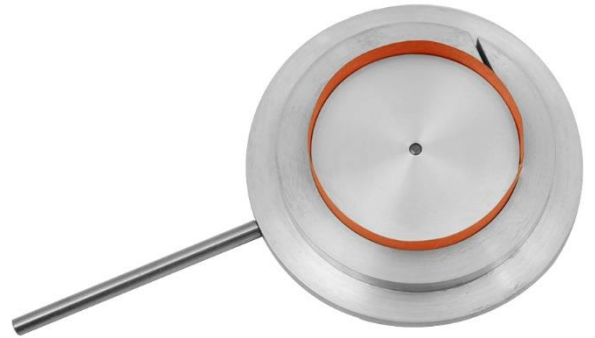
Sample holder for the Ring Crush Test (RCT)
