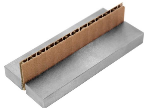
Sample holder for the Edge Crush Test (ECT)
