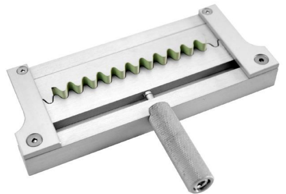
Sample holder for the Concora Crush Test (CCT)
