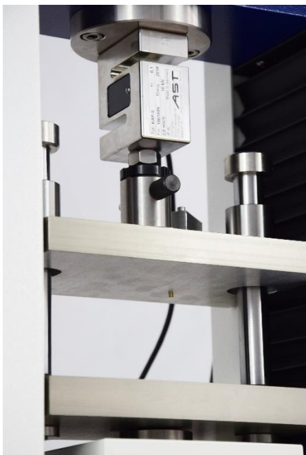
Pressure plates with frictionless guidance
