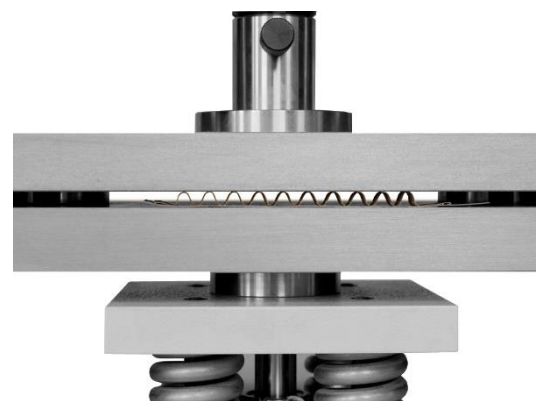
Pressure plates for the Concora Medium Test (CMT)
