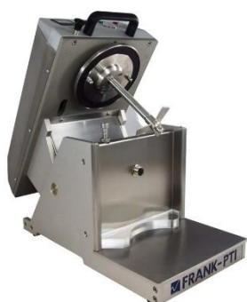
Hinged head for easy take-out of the container
