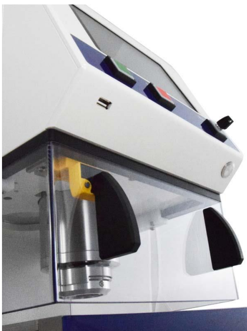
PPS with safety cover and switch
