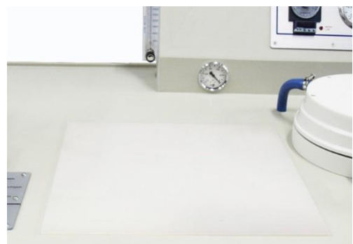
Working space with knock off plate
