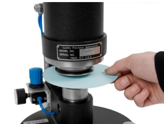
Sample is pneumatically clamped after pressing the start button
