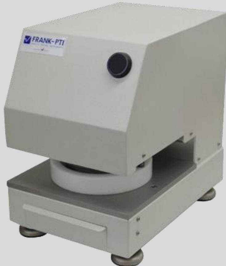
S209100003 pneumatic sample punch for grammage 100cm 2
