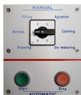
Automatic or manual control panel
