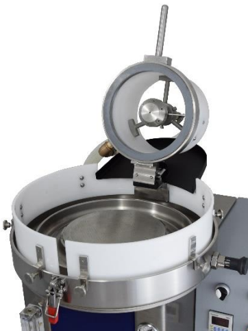
Swiveling wash chamber for quick change of sieves.
