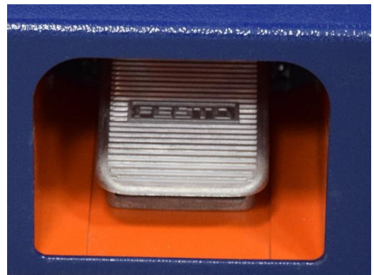
Foot pedal to activate the punching mechanism
