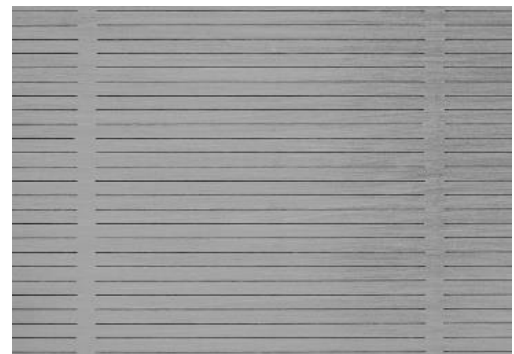
Standardized slot sieve with a slot width of 0,15 x 45mm
