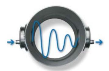
While radiating through a liquid product with microwaves they suffer a phase shift and attenuation change which directly correlates with the water content i.e. with the dry matter content of the material.
