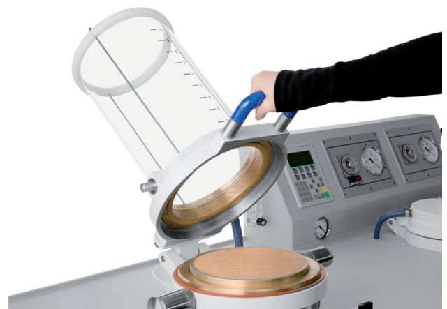
Opening the former column for taking out the hand-sheet
