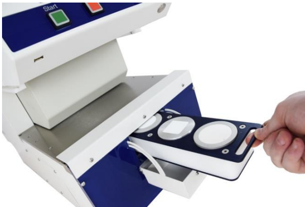
Sample stack cartridge for measuring on different grounds and for calibration on standards
