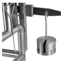
Beating pressure adjustable by use of the weight.
