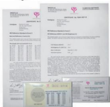
Black, white and UV standards for calibration
