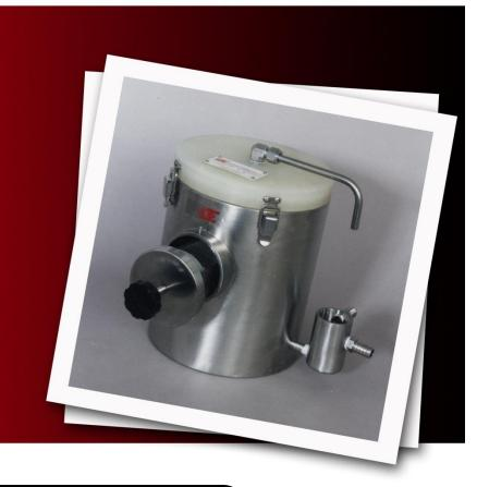
The Pulp Brightness Reversion Apparatus consists of a stainless steel vessel that holds thirty-two 25 cm<sup>2</sup> pulp specimens. The insulated vessel is heated with an external hot plate (not supplied). An internal drip roof prevents any condensation from falling onto the samples.
